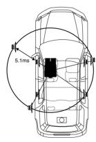
Time correction eliminates the difference between the time required for the sound from the different speakers to reach the listening position. Setting the time correction of the front left speaker to 5.1 ms makes it possible to coordinate the distance from the listening position to the speaker.
